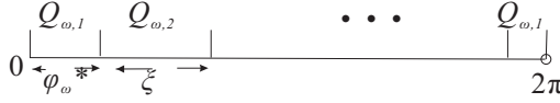
Figure 7.6: An illustration of a b -bit APQ in the phase domain, where Q_{\omega,j} , j = 1, \dots, 2^b denotes the j^{\text{th}} quantization interval with width \xi , and offset angle \varphi_{\omega}^* . The first interval Q_{\omega,1} is wrapped.
